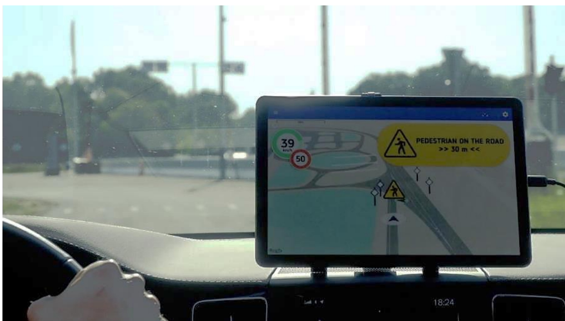
Figure 2.15: Collision alert shown on the HMI in the vehicle.
