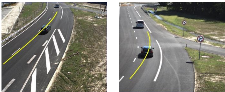
Figure 4.2: Visual tracking of the GNSS RTK antenna for evaluating the GNSS RTK accuracy (input data from May 10 th , 2019).
