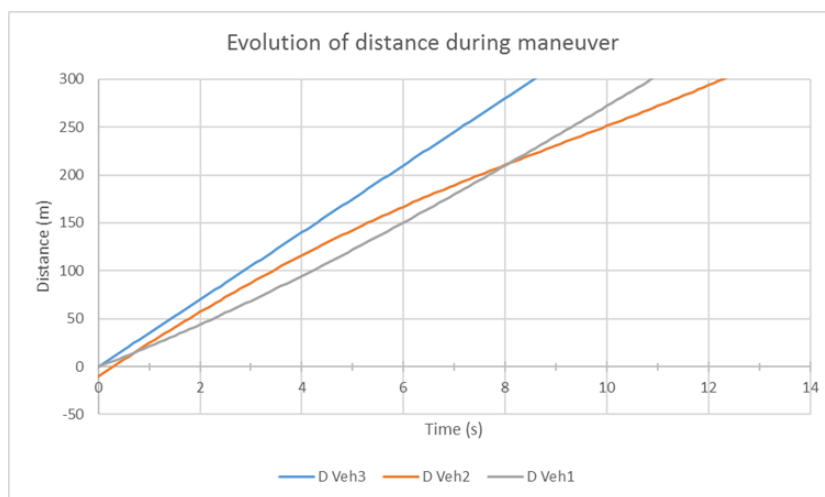
Figure 5.2: Representation of the time – distance relation between the vehicles involved in the use case
