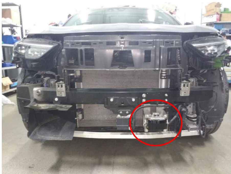
Figure 3.18: LiDAR integration in the front of the DS7.
