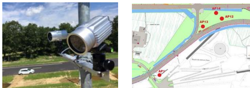
Figure 3.5: Left: two of the four cameras are mounted at 10.15 m height. Three camera streams are processed in real-time. The fourth camera serves as a backup. Right: the positions of the cameras: Camera 0 (f=8 mm) and Camera 1 (f=25 mm) on AP12, Camera 2 (f=8 mm) and backup camera on AP14.
