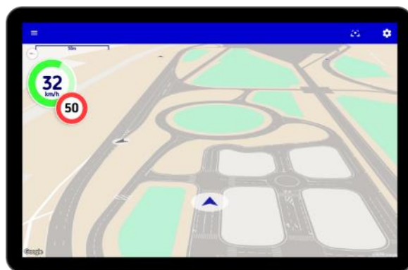
Figure 3.36: Tablet HMI on-board view.
