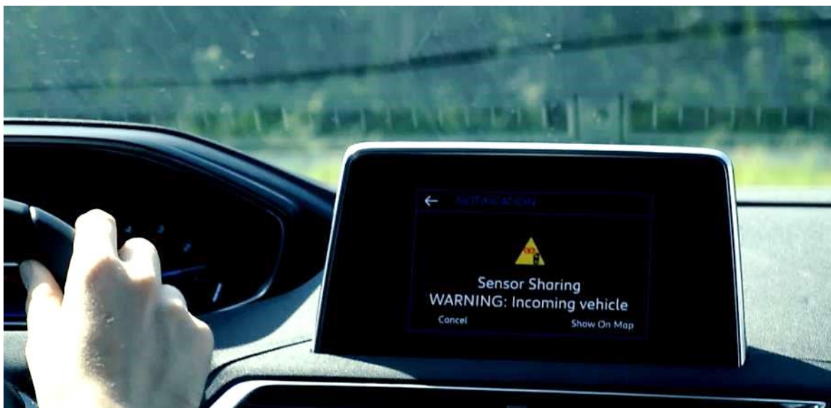
Figure 2.12: Alert message in the embedded HMI.
