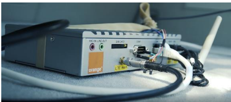
Figure 3.33: OBU in the vehicles, connected to the in-vehicle system, a rooftop antenna, and a GNSS antenna.
