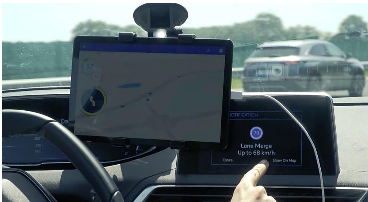
Figure 2.6: The in-vehicle HMI, as well as the tablet HMI, were used to provide warnings and instructions to the drivers.
