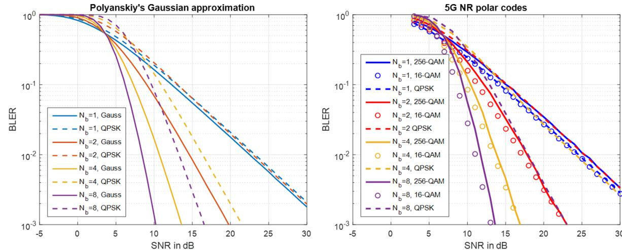
**Block error rates for transmission of 192 info bits in 128 resource elements ( $R = 1.5$  bit/use) over  $N_b$  Rayleigh fading blocks. Theoretical results (left) and 5G polar codes (right).**
