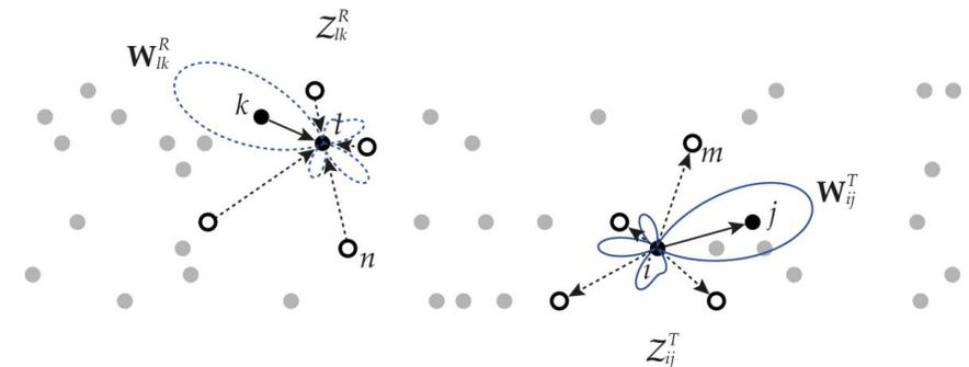
Integration of beamforming/MIMO techniques in the sidelink with BS-assisted resource allocation
