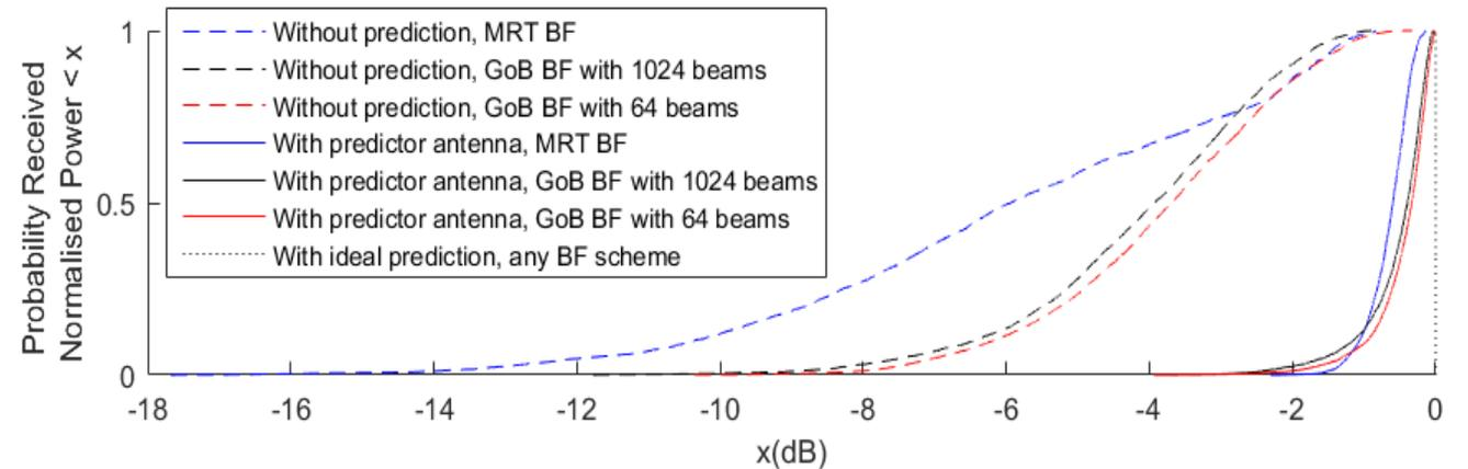
CCDF of the normalized received power metric based on practical experiments
